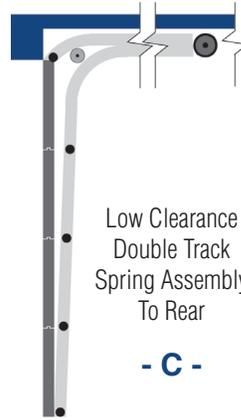
Low Clearance Double Track Spring Assembly To Rear
